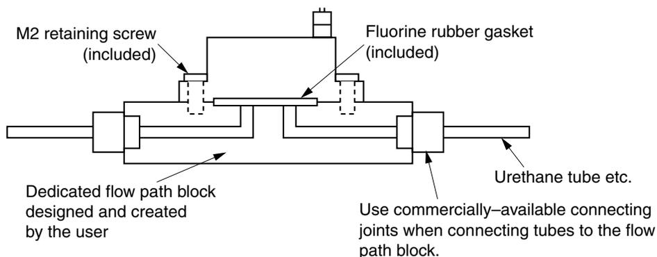
Sample composition of a flow path block unit
